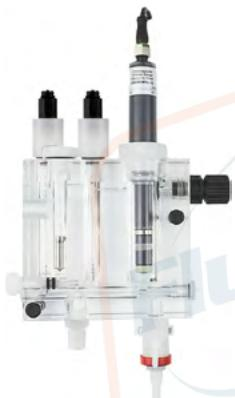
This holder is designed for the installation of a chlorine sensor Type 8232, a temperature sensor (see chapter ["8.5. Ordering chart accessories" on page 26](#)) and two electrochemical electrodes with a PG13.5 threaded connection (pH or ORP from Type 8203, conductivity from Type 8221). Further information can be found in the data sheets [Type 8232 ▶](#), [Type 8203 ▶](#) and [Type 8221 ▶](#).
