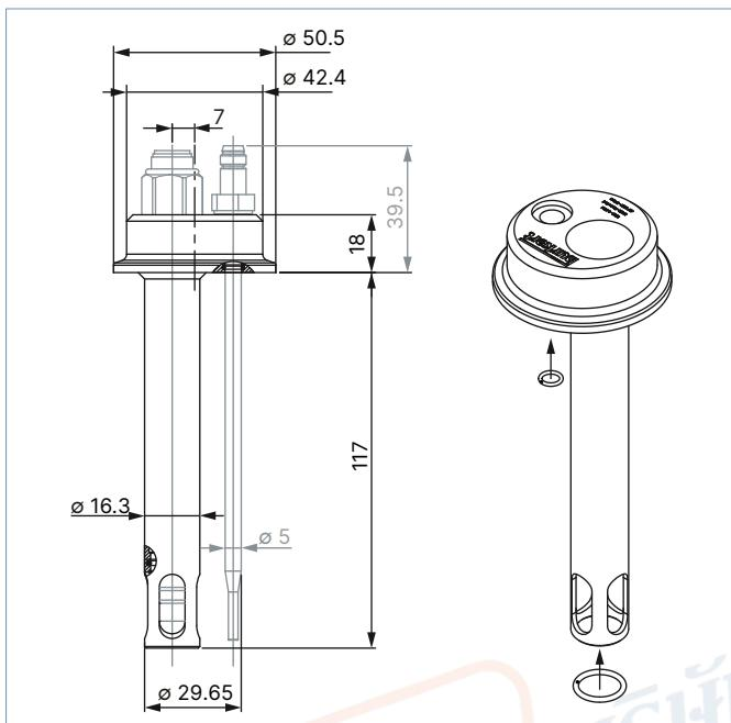
**2" (DN 50/40) connection adapted for GEA Tuchenhagen VARINLINE process connections**
