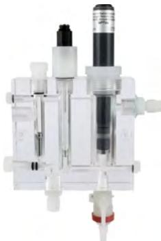
This holder is designed for the installation of a chlorine sensor Type 8232, a temperature sensor (see chapter ["8.5. Ordering chart accessories" on page 26](#)) and one electrochemical electrode with a PG13.5 threaded connection (pH or ORP from Type 8203, conductivity from Type 8221). Further information can be found in the data sheets [Type 8232 ▶](#), [Type 8203 ▶](#) and [Type 8221 ▶](#).
