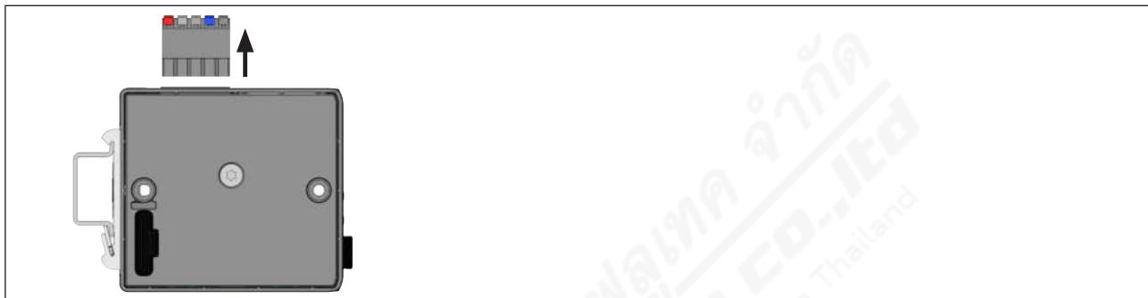
Figure 35: Remove 5-pin spring-loaded terminal
