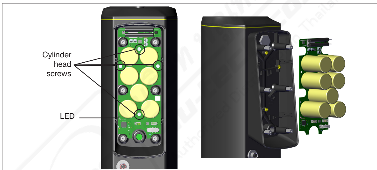
Fig. 13: Loosen screws on the printed circuit board/remove SAFEPOS energy-pack
