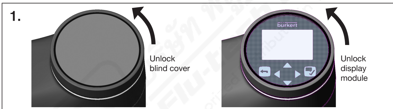
Fig. 38: Remove blind cover or display module
