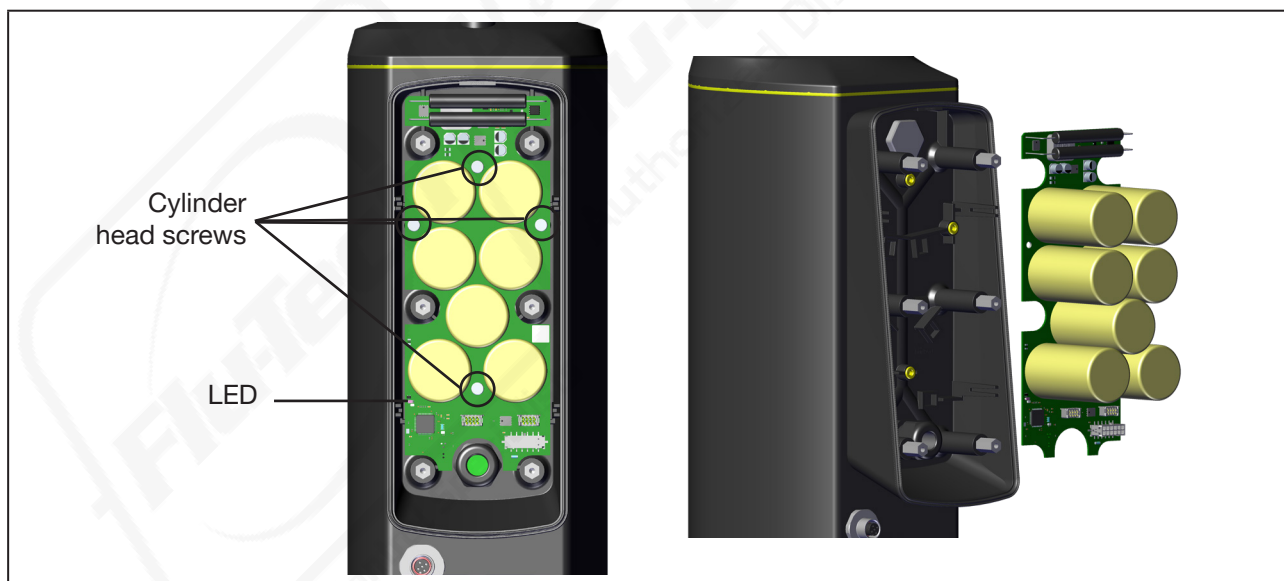
Fig. 11: Loosen screws on the printed circuit board/remove SAFEPOS energy-pack
