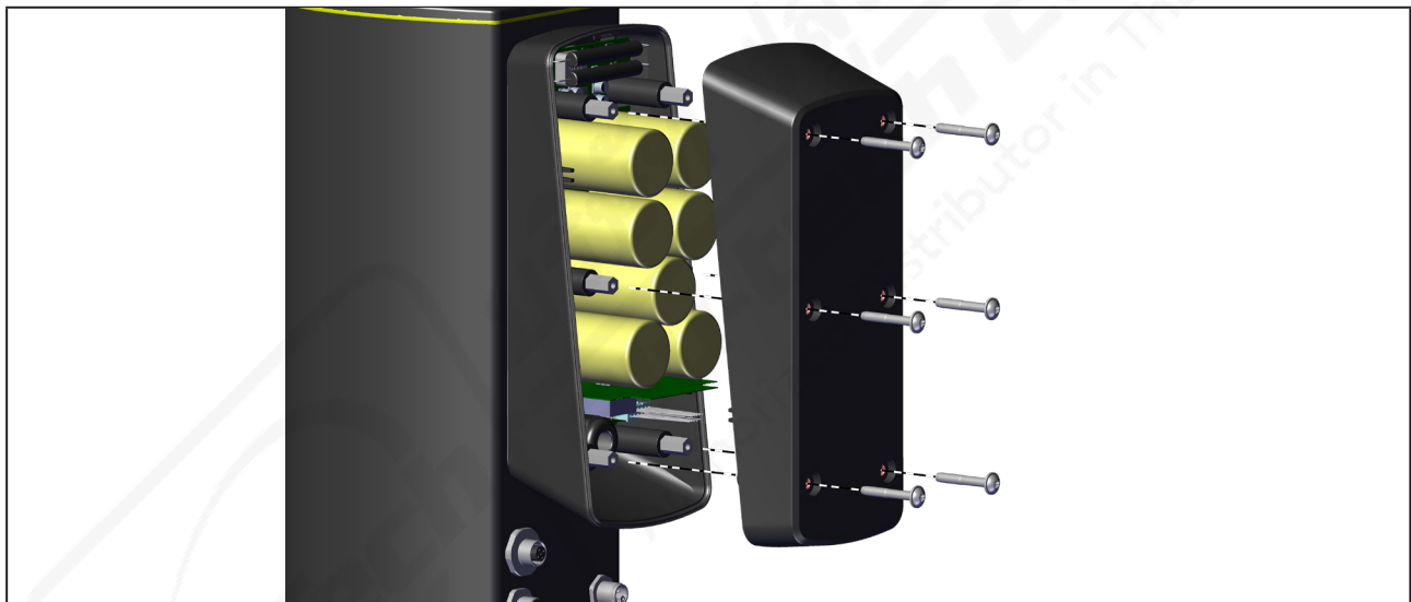
Fig. 9: Take off SAFEPOS energy-pack cover
