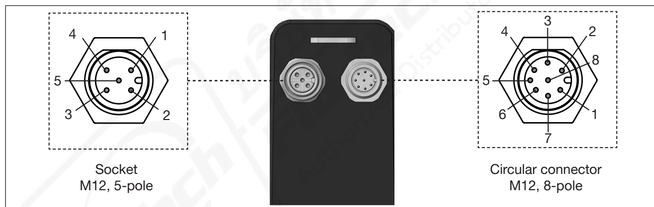
Fig. 14: Designation of the circular connector, analog version
