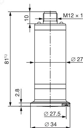
1.) The total height is increased by the height of the used female connector and cable .
