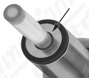
Fig 5: Gap with O ring
