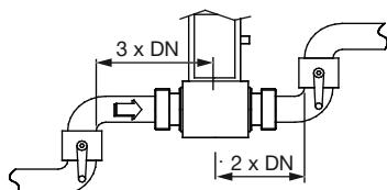
The sensor can be installed into either horizontal or vertical pipes. Mount the sensor in the below as correct indicated ways to obtain an accurate flow measurement.
