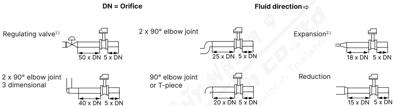
1.) If the valve cannot be mounted after the measuring device, the minimal distances have to be respected.
