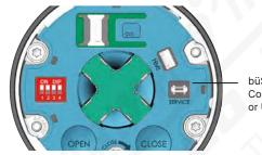
büS service interface Connection for CAN adapter or USB-büS interface set
