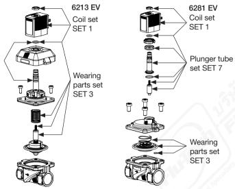
The composition of the spare part sets may differ from the diagram depending on the model of valves.
