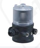
The pneumatic control units Type 8690 and 8697 are optimised for integrated mounting on process valves of the 21XX series. Mechanical or inductive limit switches detect the valve position. The integrated pilot valve controls single-acting or double-acting (Type 8690) actuators.
