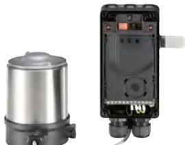
The intelligent digital positioner and process controller Type 8791/8798 is designed for mounting on linear and rotary actuators with standardisation in accordance with IEC 534-6 or VDI/VDE 3845 for demanding control tasks. The variant with remote position sensor Type 8798 is used for controlling Burkert process control valves. It is operated via a graphic display with backlight. The positioner and process controller can be initialised automatically using the TUNE functions.
