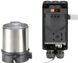
The intelligent digital positioner and process controller Type 8791/8798 is designed for mounting on linear and rotary actuators with standardisation in accordance with IEC 534-6 or VDI/VDE 3845 for demanding control tasks. The variant with remote position sensor Type 8798 is used for controlling Burkert process control valves. It is operated via a graphic display with backlight. The positioner and process controller can be initialised automatically using the TUNE functions.
