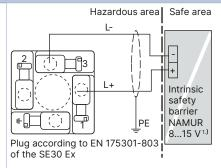
1.) Use an appropriate power supply which complies with the following electrical specifications
