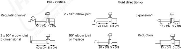
1.) If the valve cannot be mounted after the measuring device, the minimal distances have to be respected. If an expansion cannot be avoided, the minimal distances have to be respected. Please note minimum flow velocity
