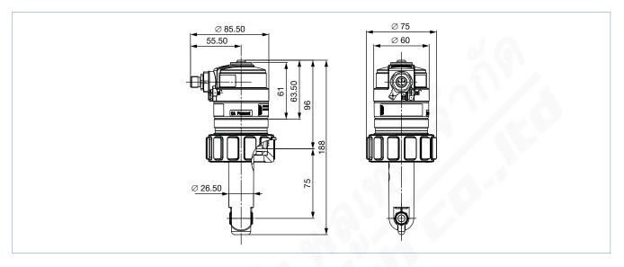
With G 2" process connection, installed in an Insertion fitting Type S020
