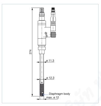
Probe with adaptation set PG 13.5 for pH armature Type 8200
