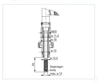
Probe with adaptation set for fitting Type 8201, welding tab DN 30 version
