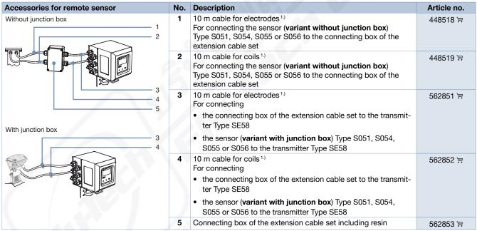
1.) Cable lengths other than 10 m on request (for cables length >20 m, a preamplifier is supplied for an additional charge).
