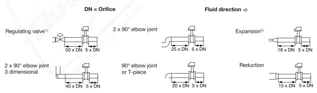
1.) If the valve cannot be mounted after the measuring device, the minimal distances have to be respected.
