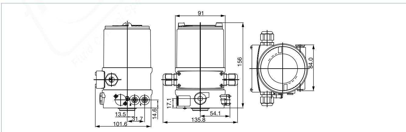
**4.3. Mounting on control valves of actuator series Type 23xx, actuator size 70/90/130/225 mm****Note:**
