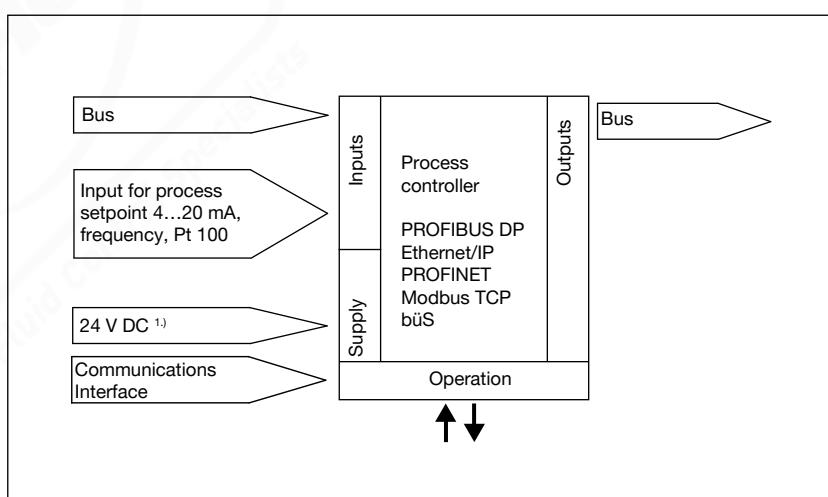
1.) The operating voltage is supplied with a 3-wire unit independent from the setpoint signal.
