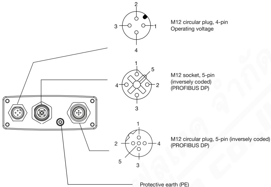
**Socket/M12 circular plug, 5-pin - fieldbus connection**
