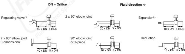
1.) If the valve cannot be mounted after the measuring device, the minimal distances have to be respected.
