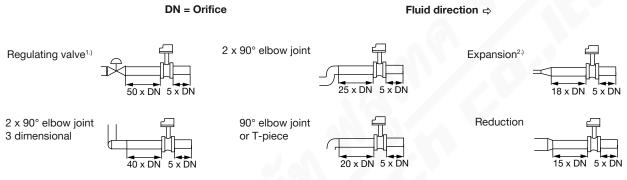
If the valve cannot be mounted after the measuring device, the minimal distances have to be respected.
