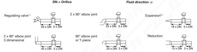
1.) If the valve cannot be mounted after the measuring device, the minimal distances have to be respected 2.) If an expansion cannot be avoided, the minimal distances have to be respected.
