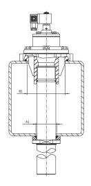
Note: Fix the valve body to the tank using the appropriate eyelets in the valve body
