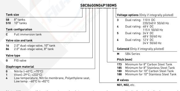
Note: When specifying the system, check temperature and pressure limits for tank, diaphragm and solenoids. Different temperature ranges maybe available, please consult your options with Pentair.
