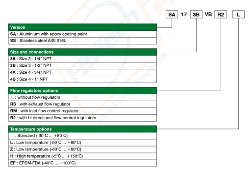
Example: SA173BVBR2L: Size 3 Volume booster, 1/2" NPT, with bi-directional flow control regulators, low temperature
