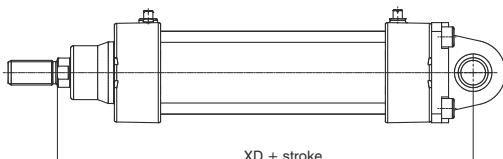
Utilised with clevis 1393.Ø.30F allows the cylinder to oscillate in all directions.
