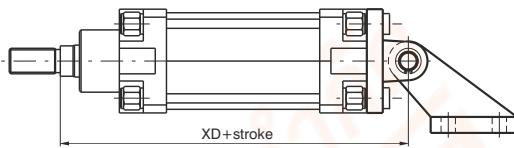
Used to mount cylinders parallel to the plane to which the counter clevis is attached. Allows self-alignment of the cylinder rod under load with an oscillation up to 90 degrees from the mounting plane.
