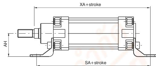
Elements used to anchor the cylinder parallel to the mounting plane. They are made of steel, and painted black.
