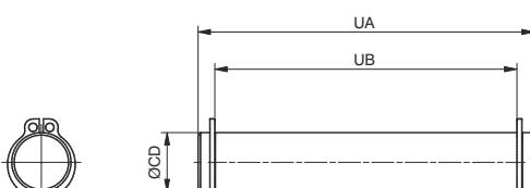
Stainless steel AISI 316 pin, complete with stainless steel circlips, which can be used with clevis code 1393.Ø.09/1F and 1393.Ø.09F
