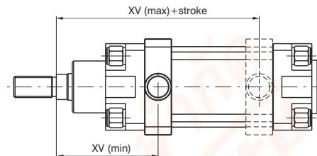
Clevis to be mounted on the barrel to have the centre of rotation of the hinge pin at a point between the end plates of the cylinder. It is attached to the barrel by means of eight pointed grains that block in the "V" groove of the four protruding shapes. In the case of anchorage subject to heavy use, it is recommended to connect the clevis once the right position has been found.
