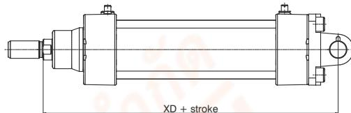
Utilised with clevis 1393.Ø.15F allows the cylinder to oscillate in all directions (see standard complete trunnion 1393.Ø.36F)
