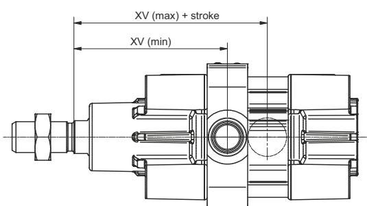
**Aluminium Intermediate Trunnion with steel bushes** to be mounted on the barrel. This solution allows the cylinder to rotate around the hinge which can be mounted in any position between the end caps. It is attached to the barrel by means of 8 grub screws which secure the Trunnion to the extruded barrel. In the case of heavy duty applications it is recommended that the Trunnion is secured using expansion pins.
