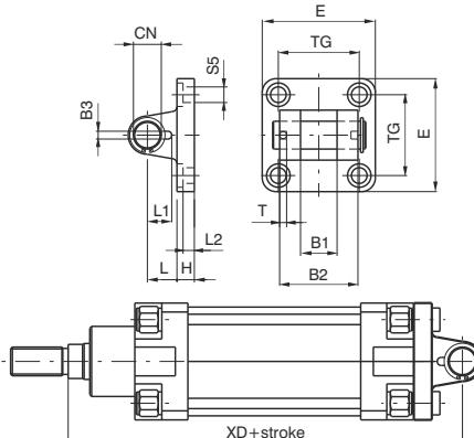
Utilised with clevis 15F allows the cylinder to oscillate in all directions. Made of aluminium alloy or steel (see ordering code) and painted black.
