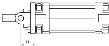
Used to mount the cylinder either parallel or at a right angle to the mounting plane; allows the cylinder to self-align under load. Made of aluminium alloy or steel (see ordering code) and painted black.
