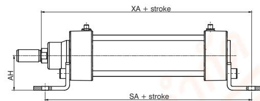
Elements used to anchor the cylinder parallel to the mounting plane. They are made of stainless steel AISI 316.
