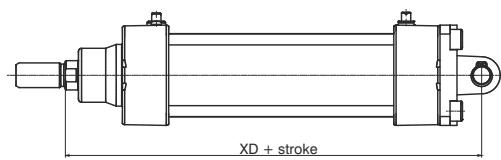
This type of mounting allows anchorage of the cylinder either parallel or right angle to plane; the cylinder rod can oscillate and self-align as necessary when under load. Made of stainless steel AISI 316.
