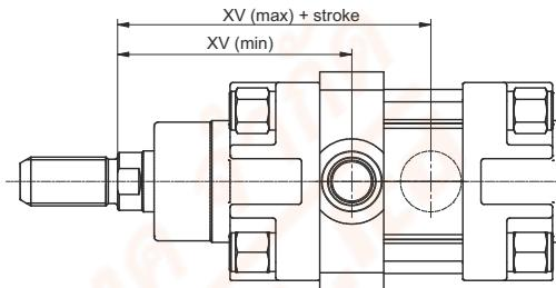
**Aluminium Intermediate Trunnion with steel bushes** to be mounted on the barrel. This solution allows the cylinder to rotate around the hinge which can be mounted in any position between the end caps. It is attached to the barrel by means of 8 grub screws which secure the Trunnion to the extruded barrel. In the case of heavy duty applications it is recommended that the Trunnion is secured using expansion pins.
