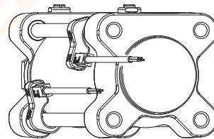
To mount the brackets on the tie rods use the dedicated stainless steel grub screw.
