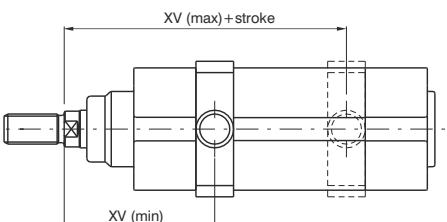
Clevis to be mounted on the barrel to have the centre of rotation of the hinge pin at a point between the end plates of the cylinder. It is attached to the barrel by means of eight pointed grains. In the case of anchorage subject to heavy use, it is recommended to connect the clevis once the right position has been found.
