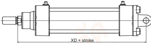
Similar to 09 clevis except for the connection, which is male rather than female. Used to mount the cylinder either parallel or at a right angle to the plane; the cylinder rod can oscillate and self-align as necessary when under load. Made of stainless steel AISI 316.
