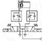
System to stop the cylinder on intermediate position with higher tolerances.
