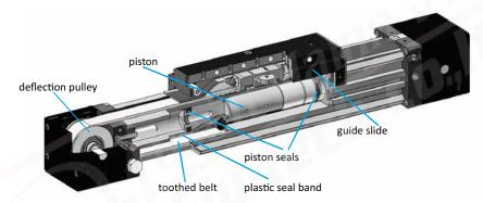
In the outer chamber, the piston bracket grips the toothed belt, which leads to a tension lock at the opposite side via the deflection pulley. Inside the slide, the cover belt is lifted from the slot, and the slide is connected to the tension lock.
