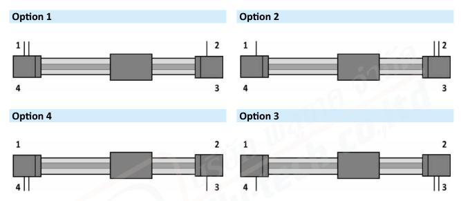
The cylinder is supplied with three air connections. Two connections are necessary for operation, while the third is closed by a plug (included in the scope of delivery). The desired position of the double connection has to be specified in the order code after the stroke length by choosing the adequate number.
