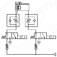
This control circuit improves the positioning accuracy. The use of check valves reduces the stopping distance and also increases the load stiffness.
