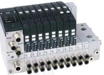
Manifold system with integrated electrical connection including LED indicators. Each station can accommodate two 3/2-way valves or one 5/2- or 5/3-way valve. All connections are accessible from the front.
