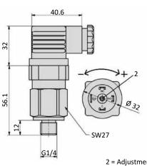
2 = Adjustment of pressure range (with hex key 1,5 mm)
