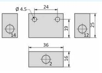
12, 14 = signal input = signal output
