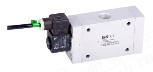
Electrically operated valves conform to equipment category 2 can be used in Zone 1 respectively in Zone 21. For the use in hazardous areas the category group of the used coil has to be taken into account. The specification of the whole equipment corresponds always to the lowest category of the single components.
