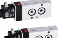
Electrically operated spool valve. The manual override is detent and is operated by screw driver. The model KN-55 has a coil with enhanced humitidy resistance and a additional gasket at the coil. The location pin, screws and seals are included.
