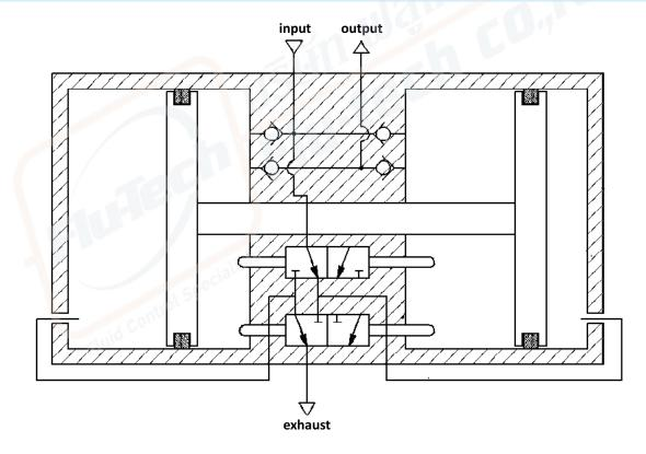
The Pressure booster 90-PB is suitable only for compressed air.
