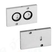
Converting plate suitable to obtain a 3/2-way function at a 5/2-way NAMUR valve. Additional feature: Turning the plate by 180° you can change a NC to a NO function or vice versa.
