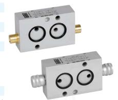
Flow control valves for speed regulation of pneumatically operated actuators. Mounting between NAMUR valve and actuator. Adjustable with screwdriver or manually. The location pin, screws and seals are included.
