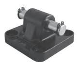
Similar to 09 clevis except for the connection, which is male rather than female. Used to mount the cylinder either parallel or at a right angle to the plane; the cylinder rod can oscillate and self-align as necessary when under load. Made of aluminium alloy or steel (see ordering code) and painted black.
