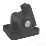
Mounting consists of clevis 09 and counter clevis. Used to mount cylinders at a right angle to the plane to which the counter clevis is attached. Allows self-alignment of the cylinder
