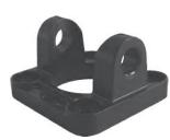
Used to mount the cylinder either parallel or at a right angle to the mounting plane; allows the cylinder to self-align under load. Made of aluminium alloy or steel (see ordering code) and painted black.
