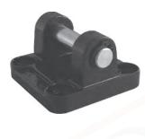
Similar to type 08 but includes a hinge pin. This type of mounting allows anchorage of the cylinder either parallel or right angle to plane; the cylinder rod can oscillate and self-align as necessary when under load. Made of aluminium alloy or steel (see ordering code) and painted black.
