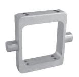
Clevis to be mounted on the barrel to have the centre of rotation of the hinge pin at a point between the end caps of the cylinder. It is attached to the barrel by means of eight pointed grains. In the case of anchorage subject to heavy use, it is recommended to connect the clevis once the right position has been found.
