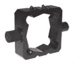
Aluminium Intermediate Trunnion with steel bushes to be mounted on the barrel. This solution allows the cylinder to rotate around the hinge which can be mounted in any position between the end caps. It is attached to the barrel by means of 8 grub screws which secure the Trunnion to the extruded barrel. In the case of heavy duty applications it is recommended that the Trunnion is secured using expansion pins.
