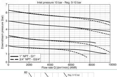
Pressure regulator Stainless steel line have been designed to withstand a 60 Bar maximum inlet pressure.
