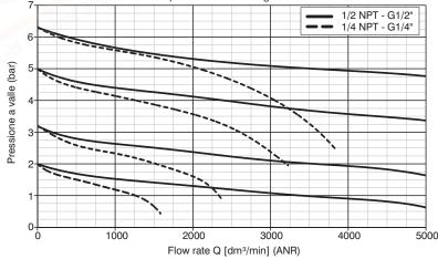
Pressure regulator Stainless steel line have been designed to withstand a 60 Bar maximum inlet pressure.
