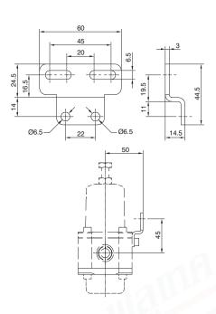
Weight 32 gr. AISI 316L stainless steel material. Allows wall fixing of individual products.
