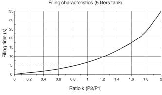
P1 = inlet pressure P2 = tank pressure
