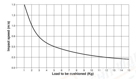
In case of extreme applications close to the maximum allowed values in the graph it is strongly recommended to ad external damping systems.
