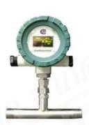
Available in 12V<sub>DC</sub>,24V<sub>DC</sub>, 115-230V<sub>AC</sub> (2.5W)
