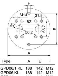
GPD06 KL GPD06 188 142 M12 Connecttions only for bottom entry. metric threads А Type
