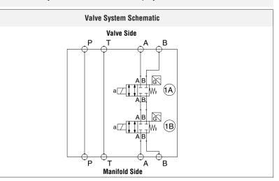
The HDBH Series system is a redundant, dual blocking valve system designed for critical applications where safe stopping is required for hydraulically controlled actuators. This valve system is equipped with inductive position switches for external monitoring by an electrical safety control system. The HDBH valve is designed to be sandwich-style mounted (interposed) between a manifold and a directional valve, or in-line mounted by use of optional mounting kits.
