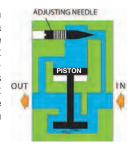
When inlet pressure is removed, downstream air is exhausted through the inlet port and around the point of the adjusting needle.
