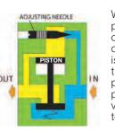
When downstream pressure reaches a certain percentage of inlet pressure, it is enough to actuate the valve's piston and the inlet poppet opens. The valve is now open to full air flow.
