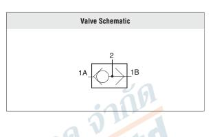
ROSS shuttle valves or double check valves have two inlets and one outlet. The first inlet to be pressurized is connected to the outlet, and the second inlet is then closed. Thus, a pneumatic device connected to the shuttle outlet can be operated by either of two control valves connected to the shuttle inlets. Automatically blocks one inlet passage when pressure is applied to the second inlet. Pressure to either inlet is channeled to one outlet port.
