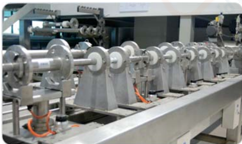
Piping system I (Max capacity for four meters calibration simultaneously in above system.)
