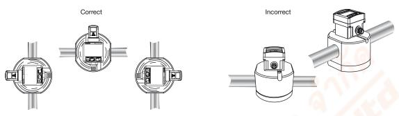
The pipe must be filled with liquid and free from air bubbles. Avoid air purge of the system which would cause damage and to prevent damage from dirt or foreign matter, we strongly recommend the installation of a 250 µm strainer as close as possible to the inlet side of the meter.
