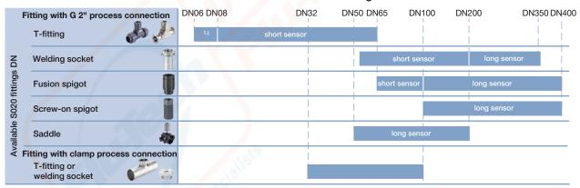
1.) DN06 and DN08: S020 in stainless steel only and 8041 with stainless steel sensor recommended
